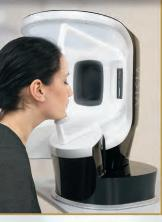
VISIA's capture module rotates around the stationary subject to capture left, right and frontal facial views.
